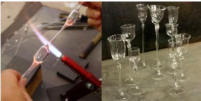
**Lampworking with borosilicate glass**
